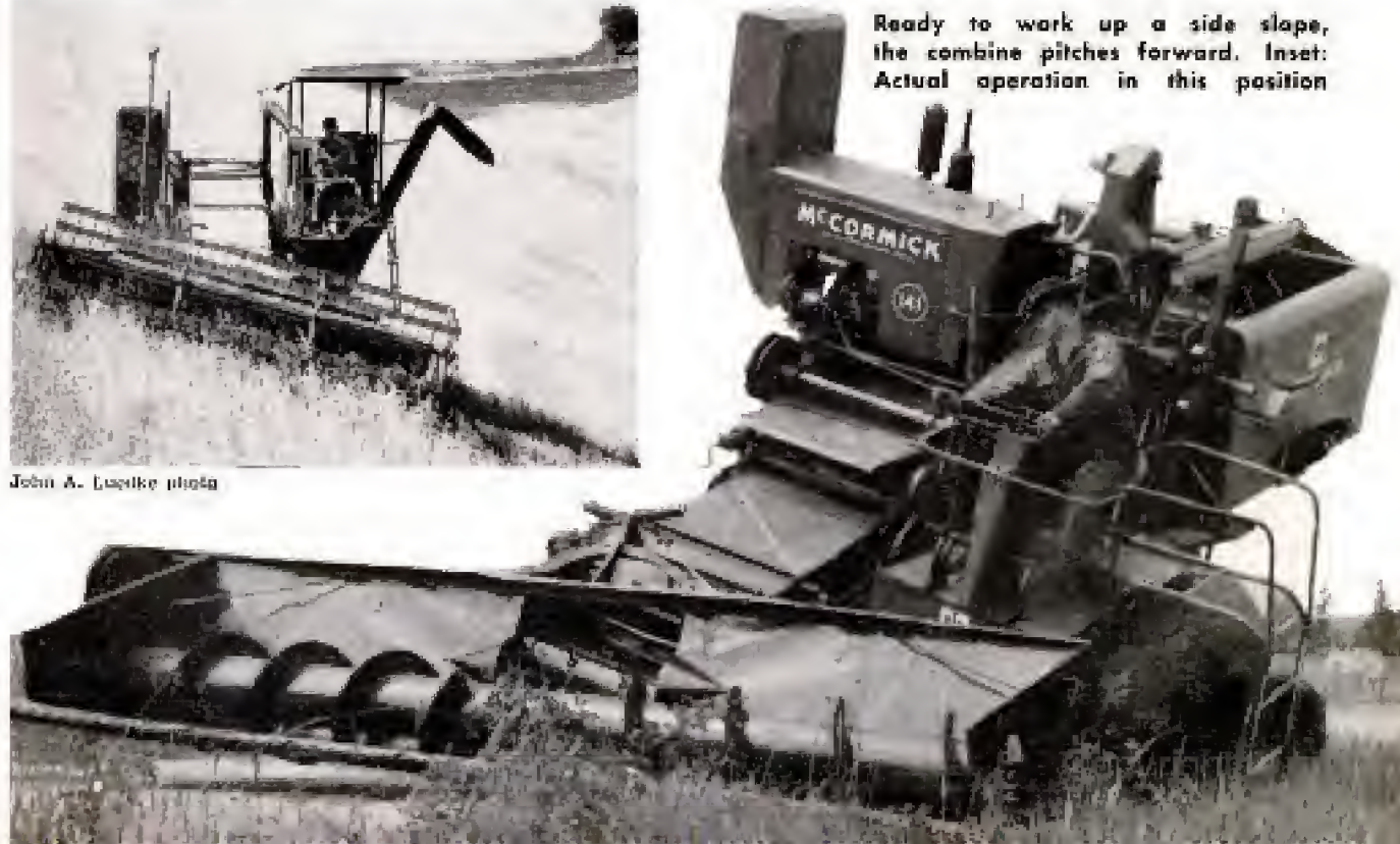
The combine can adjust for any contour. Here it is set to work down a hill that slopes to the left.
